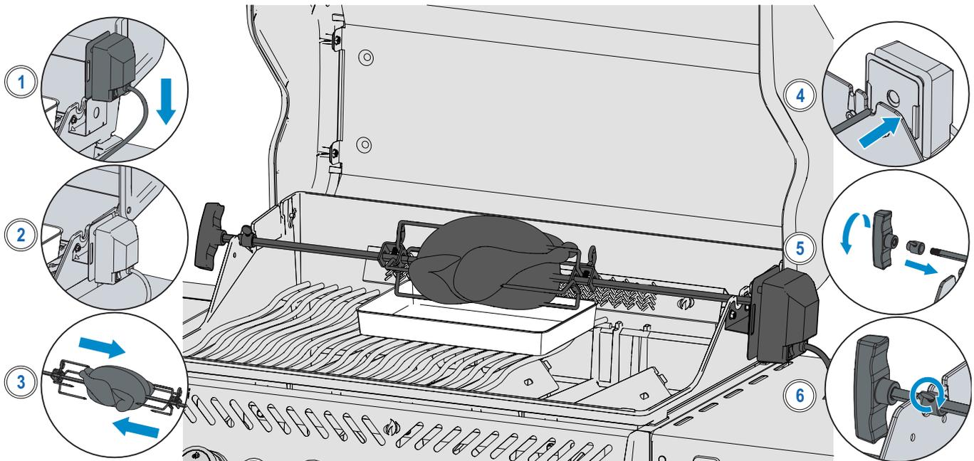
Ensure stop bushing is tightened on the inside of hood casting.
